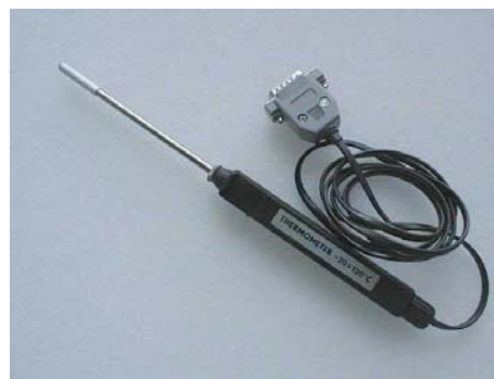
Figure 1 Thermometer; range -20 \text{ }^{\circ}\text{C} \div +120 \text{ }^{\circ}\text{C} .
