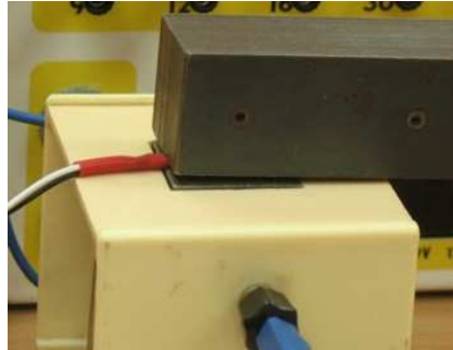
Fig. 2: Detail of the Hall's probe inside the gap of the transformer's core (to measure the dependence of B on I )
