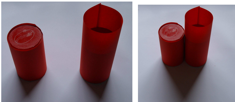
Figure 9: Shadows of two cylinders with the same cross section and different height. The triangular shadows are the same. On the right photo, these two cylinders are put next to each other. The shadow is still triangular. We conclude that the height of the object does not influence the height of the triangular shadow.
