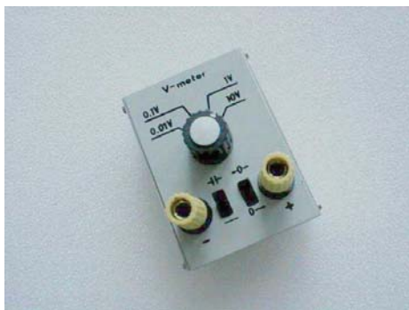
Figure 1. V-meter; range 10 \text{ mV} \div 10 \text{ V} .
