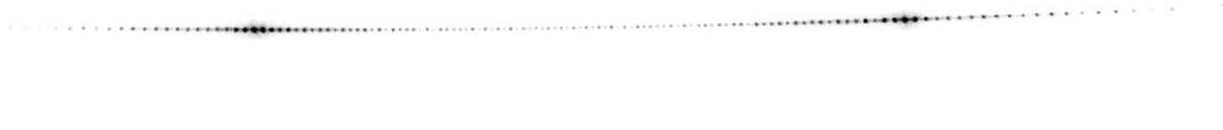
Figure 6: Pattern obtained on the screen when laser beam is incident perpendicularly to the foil in forward direction. The photography has been inverted.
