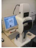
Figure 3. SMI HighSpeed eye tracker.
