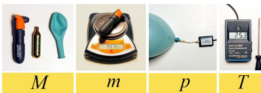
Figure 1. Equipment needed to perform the experiment (from left to right): bicycle inflator, CO 2 cartridge, balloon, precision scales, gas sensor and thermometer.
