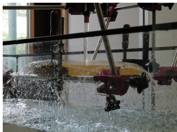
Figure 6: Water jet meets watchglass, initial experimental set-up.
