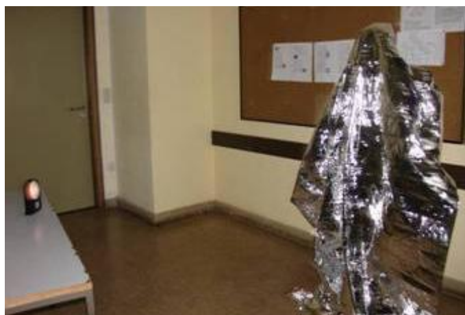
Fig. 3: An experiment: Trying to "outfox" an infrared motion detector (covering infrared radiation).
