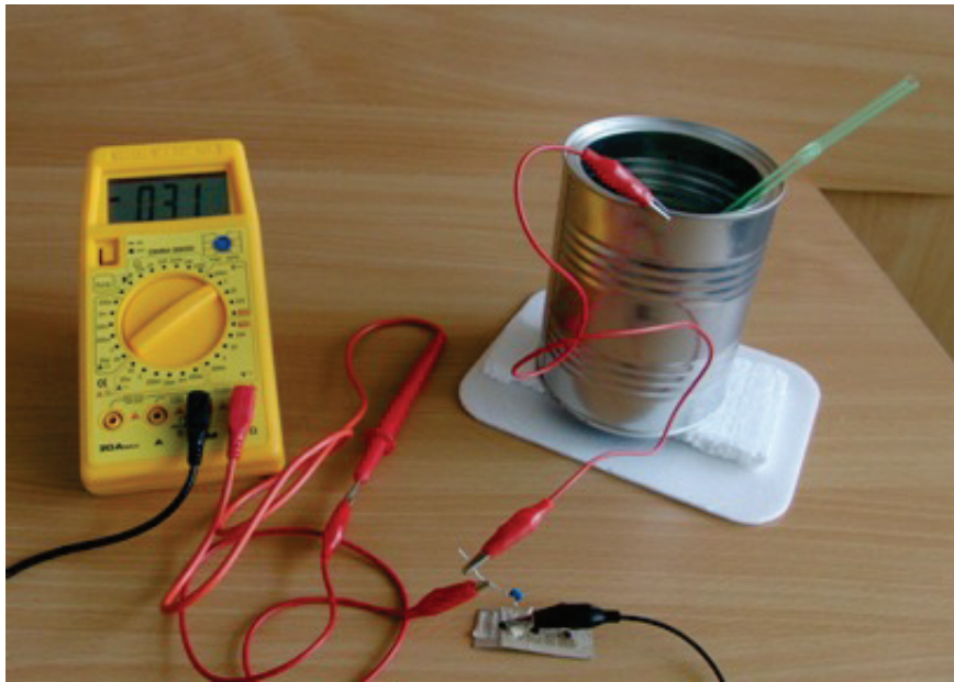
Fig. 5. The real measurement of a charge by a capacitor and an ordinary multimeter
