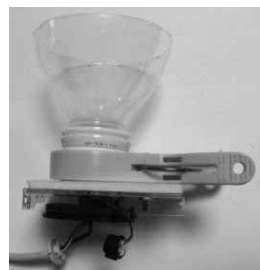
Fig. 4 USB Camera for Plastic Bottle Microscope.
