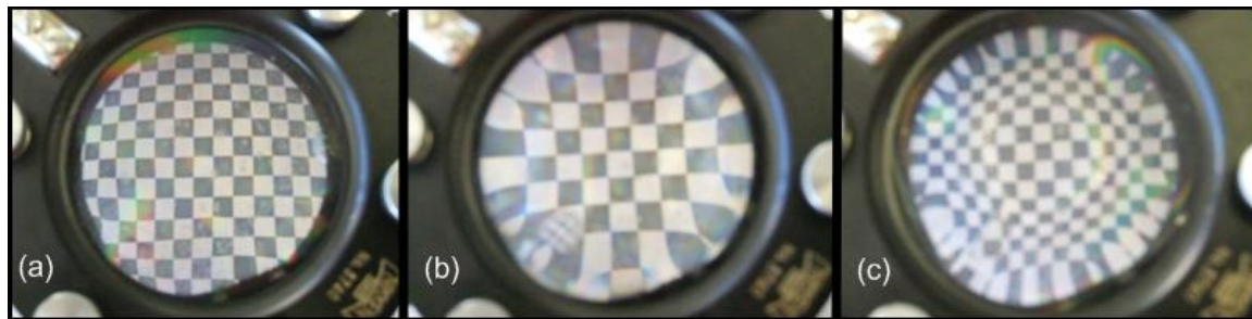
Figure 5. Focusing a chessboard pattern with a liquid filled lens. The lens is flat ( \Delta V = 0 ) in (a), biconvex ( \Delta V > 0 ) in (b) and biconcave with a flat central region ( \Delta V \ll 0 ) in (c). The aperture of the lens is 50 mm and the thickness of a flat lens in (a) is 5 mm.
