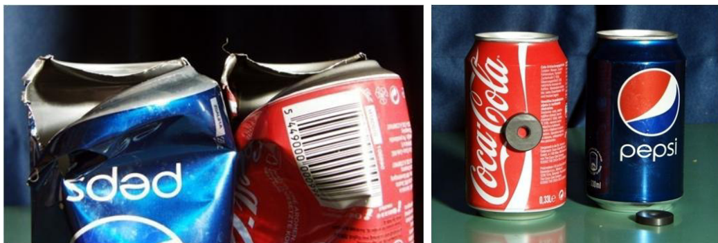
Figure 4. Thicknesses of the can bottoms are equal (left). A magnet sticks to the Coke can but does not stick to the Pepsi can (note: in some parts of Europe and Asia about half of soda cans are made from steel and other half from aluminium.)
