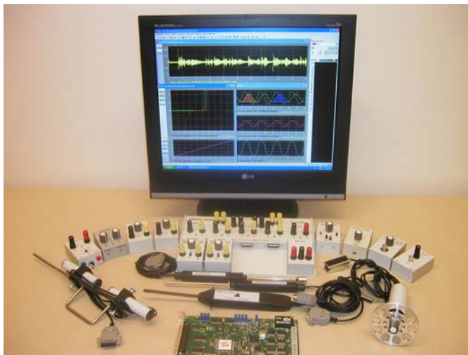
Figure 1. Internet School Experimental System (ISES): Hardware with the main panel, interface card and incomplete set of modules.
