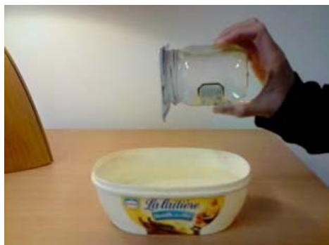
Figure 7. In a horizontal position, the water also does not flow out of the glass
