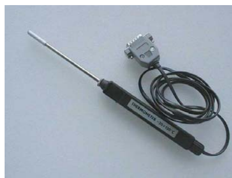
Figure 1 Thermometer; range -20 \text{ }^\circ\text{C} \div +120 \text{ }^\circ\text{C} .
