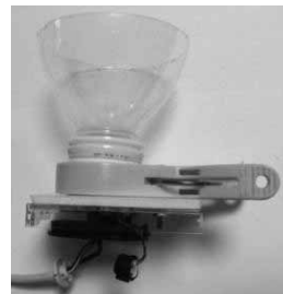
Fig. 4 USB Camera for Plastic Bottle Microscope.
