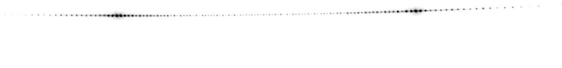
Figure 6: Pattern obtained on the screen when laser beam is incident perpendicularly to the foil in forward direction. The photography has been inverted.
