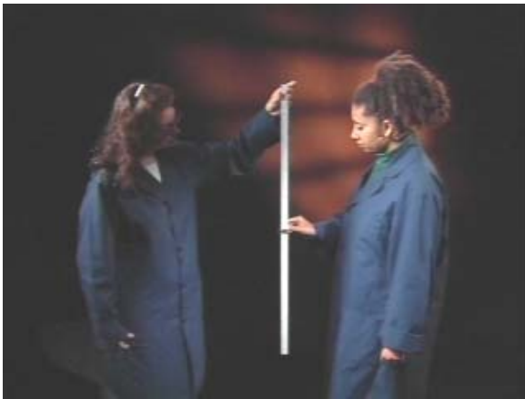
Fig. 2: Example of a “tangible” to measure human reaction time. By dropping the meter stick from a fixed position, the time needed to catch the falling stick can be deduced by a direct measurement of the free-fall distance.
