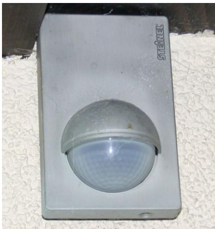
Fig. 3: An experiment: Trying to "outfox" an infrared motion detector (covering infrared radiation).
