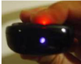
Fig. 1. “Seeing” through a camera IR radiation emitted by a remote control
