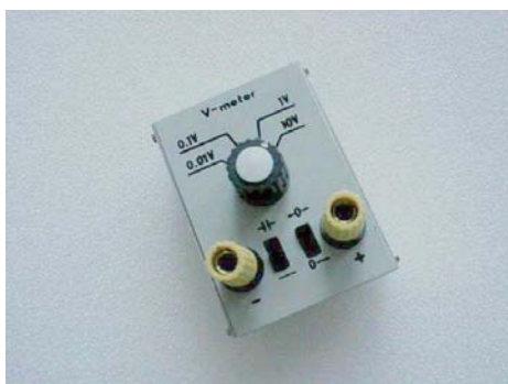
Figure 1. V-meter; range 10 \text{ mV} \div 10 \text{ V} .
