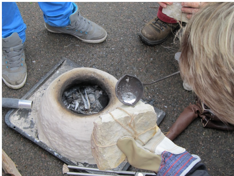
Figure 3. Tin casting in tufa
