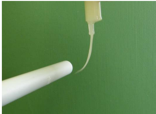
Figure 3. Homemade ER fluid jet close to a charged ebonite rod
