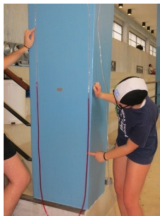
Figure 1. Measuring the equivalent pressure generated by our respiratory system with a U-manometer
