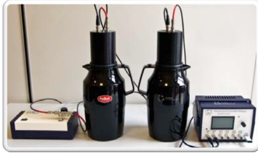
Figure 1. One set of the “coffee pot” experiment with a power supply, two coffee pots filled with water, two photomultipliers screwed on top and a data box
