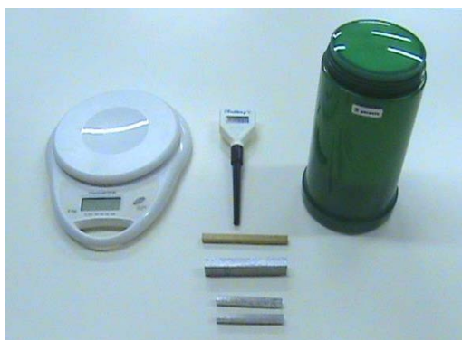
Figure 1. A balance, a digital thermometer, a Dewar vessel and various metal bars were utilized for investigating thermal equilibrium
