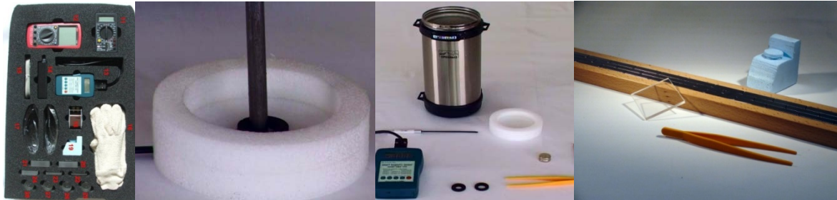
Figure 1. The HTK of the project Mosem and some examples of materials for Meissner effect, magnetic levitation, MAGLEV model [17-18].
