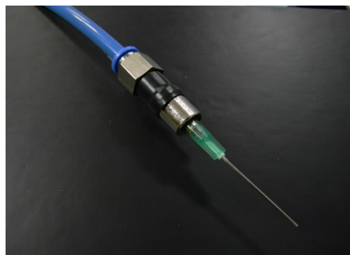
Figure 4. Improved connection to support higher air pressures and avoid leaks
