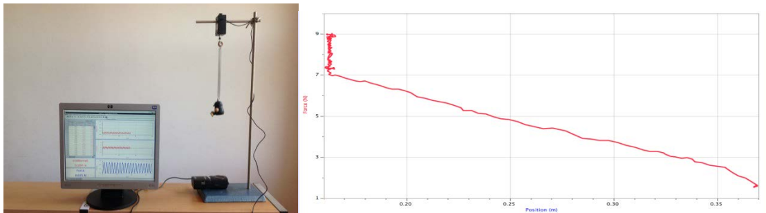
Figure 8. Force-position dependence taken by the Vernier Go!Motion sensor and DualRange Force sensor. Left – arrangement of the experiment, right – plot of the collected data.
