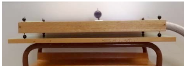
Figure 2. The bouncing disk on an air table, it is well visible the target object (black ball)
