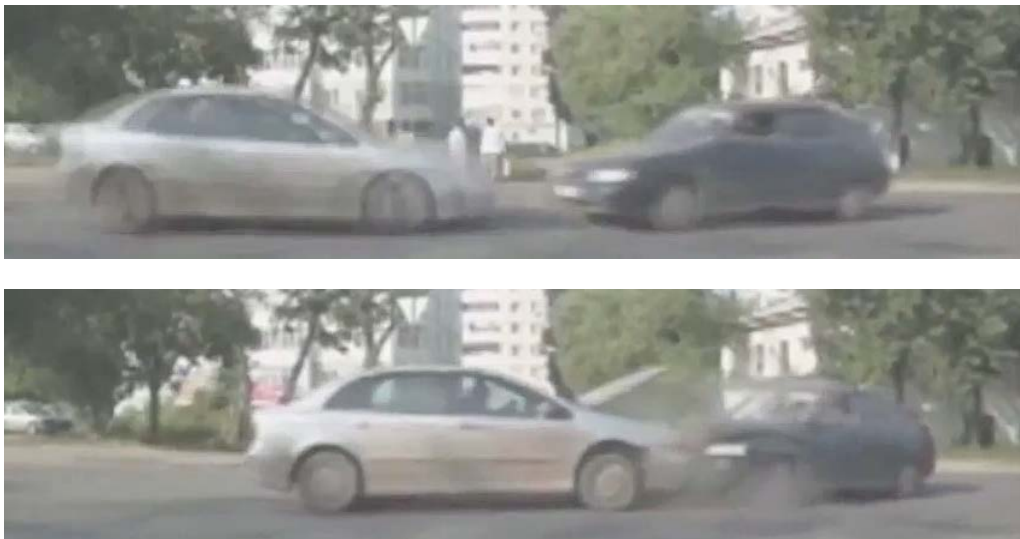
Figure 2. Video frames of two cars undergoing a head on collision
