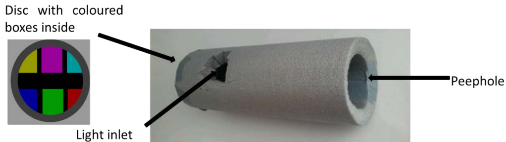
Figure 3. The Colour Vision Tube (CVT)
