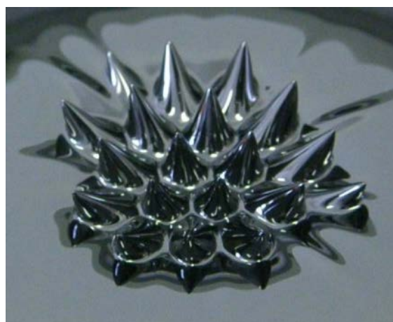
Figure 10. The surface of a ferrofluid in the presence of an external magnetic field
