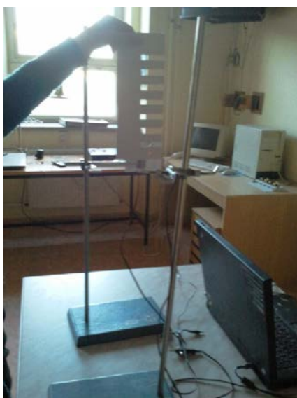
Figure 2. Free fall of a paper comb
