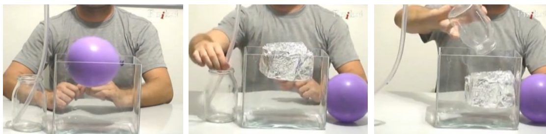
Figure 1. Balloon floating on gas (left), boat floating on gas (centre) and boat sinking after it is filled with gas (right); frames from educational video accessible at http://www.fizik.si/index.php/en/fizikalni-eksperimenti/mehanika?videoid=xQo-v_F1P9U#youtubegallery
