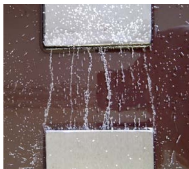
Figure 2. Scattered ground grain on a layer of oil, in the presence of high voltage
