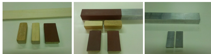
Figure 3. Surfaces proposed in the inquiry-based exploration on sliding friction: wood, sandpaper and steel.
