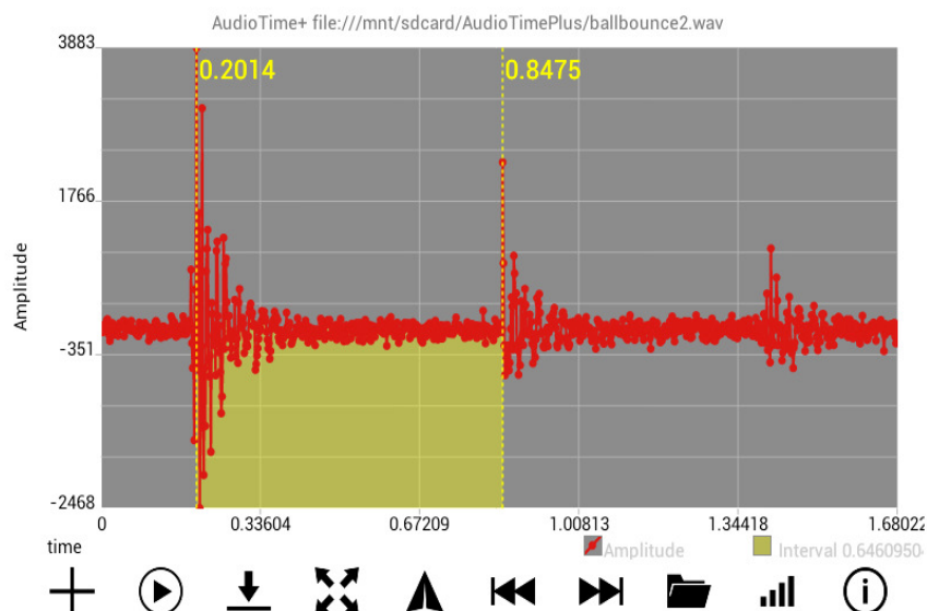
Figure 7. The sound of a ball bouncing three times as recorded by our sound app. A very accurate measurement of the time between bounces can be made from the recorded sound.
