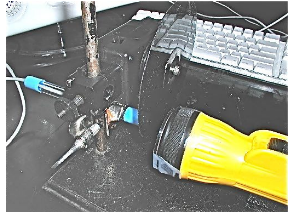
Figure 8. Computer-based apparatus used to analyze polarized light.
