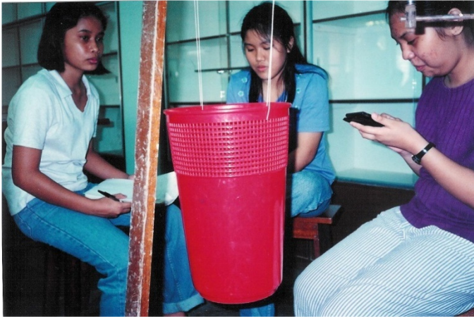
Figure 2: Rotation pendulum in the Philippines. Weights could be placed closer or farther from the center, strings could be lengthened/shortened, the basket could be changed.
