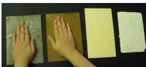
Figure 4. Arranging plates made of various materials from the coldest to the warmest.
