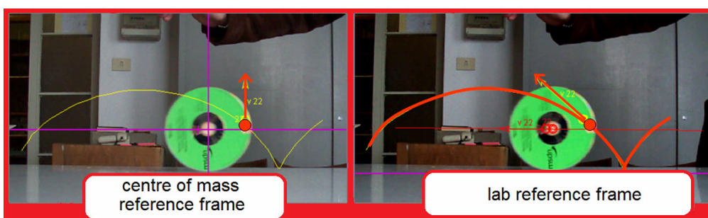
Figure 1. In the snapshot the velocity vectors in the centre of mass and lab reference frames of a point on the edge of the disk are shown at the same instant.
