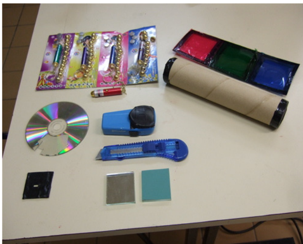
Figure 16. Low cost equipment used in ALOP: inexpensive lasers, diffraction gratings from discarded CDs, slits scratched into coated mirrors, cellophane color filters and spectrometer made from a diffraction slide.
