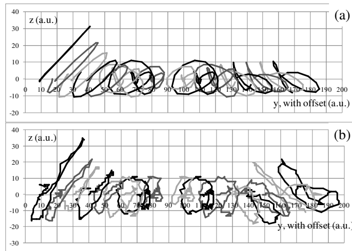
Figure 6. Comparison of polarization for an initial 45^\circ pulse. (a) values calculated via Fourier transforms vs. (b) measured values. The two components of displacement are denoted z and y and are plotted for the duration of the pulse at that position along x . The y component is offset to indicate where along the x axis a particular polarization occurs.
