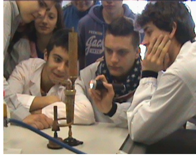
Figure 1. Students during the measurement of the alcoholic strength of a solution by using the Malling ebulliometer.
