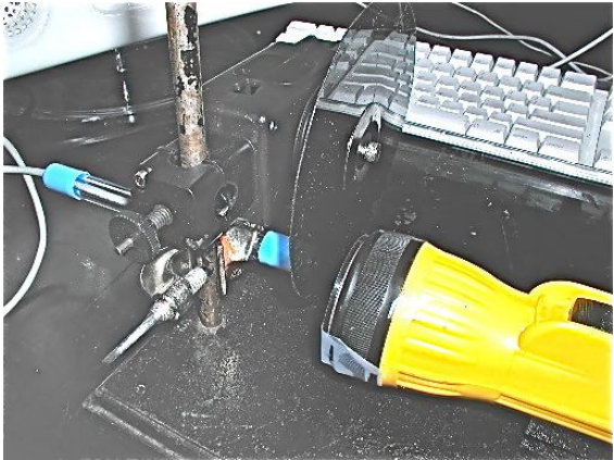
Figure 8. Computer-based apparatus used to analyze polarized light.
