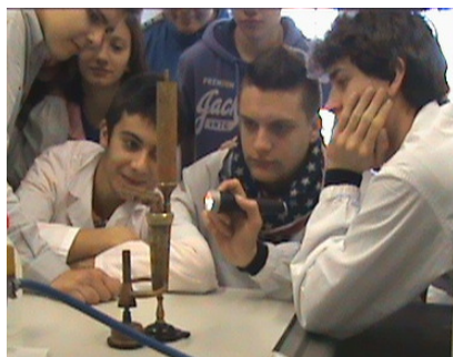
Figure 1. Students during the measurement of the alcoholic strength of a solution by using the Malligand ebulliometer.
