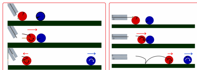
Figure 6 Shots with top or bottom spin and consequences on the motion after the collision.
